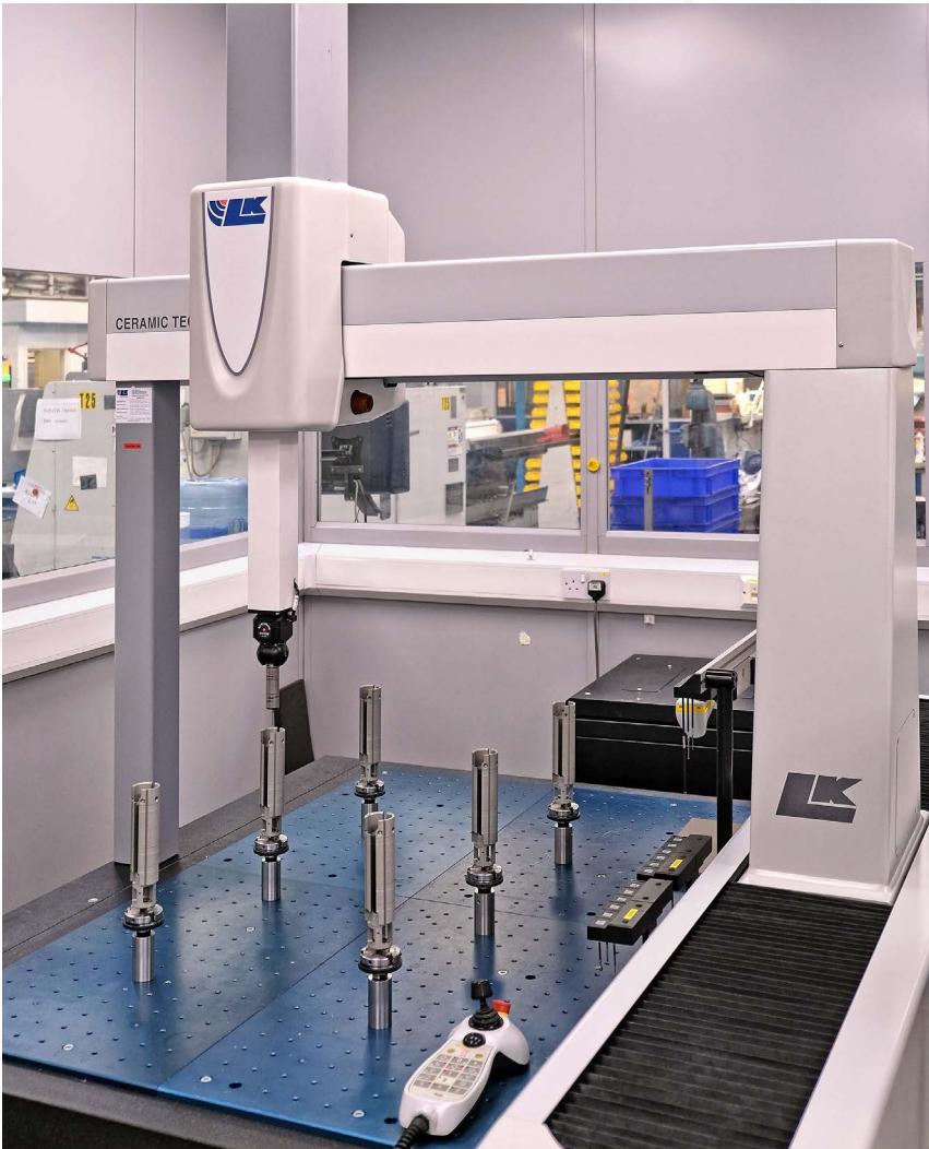
Six hard anodised aluminium oil exploration components, batch loaded onto the table of the LK AlteraS 15.10.8. Up to 12 smaller components may be placed on the table with the help of permanently located, pre-drilled fixture plates attached to the granite. This machine, and its smaller counterpart at Wilford, has a specification that includes accuracy starting at 1.8 µm + L/400, a repeatability of 1.7 µm, and speed and acceleration of 762 mm/sec and 2,306 mm/sec 2 respectively.
