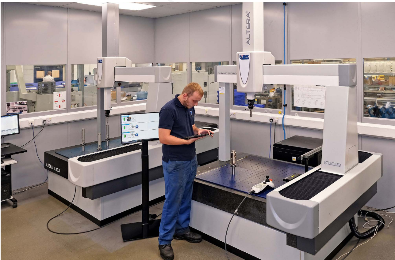
A machinist in the inspection room at Wilford at the end of a measuring cycle on a Nibron (high-strength cupronickel) component that he was previously responsible for loading onto the LK AlteraS 10.10.8 with the help of Launchpad (seen on the screen to the left). Results are displayed on his networked tablet and may also be called up on the static screen. The software will shortly be enhanced to include functionality that allows the operator on the shop floor to be alerted when a measuring cycle is complete.
